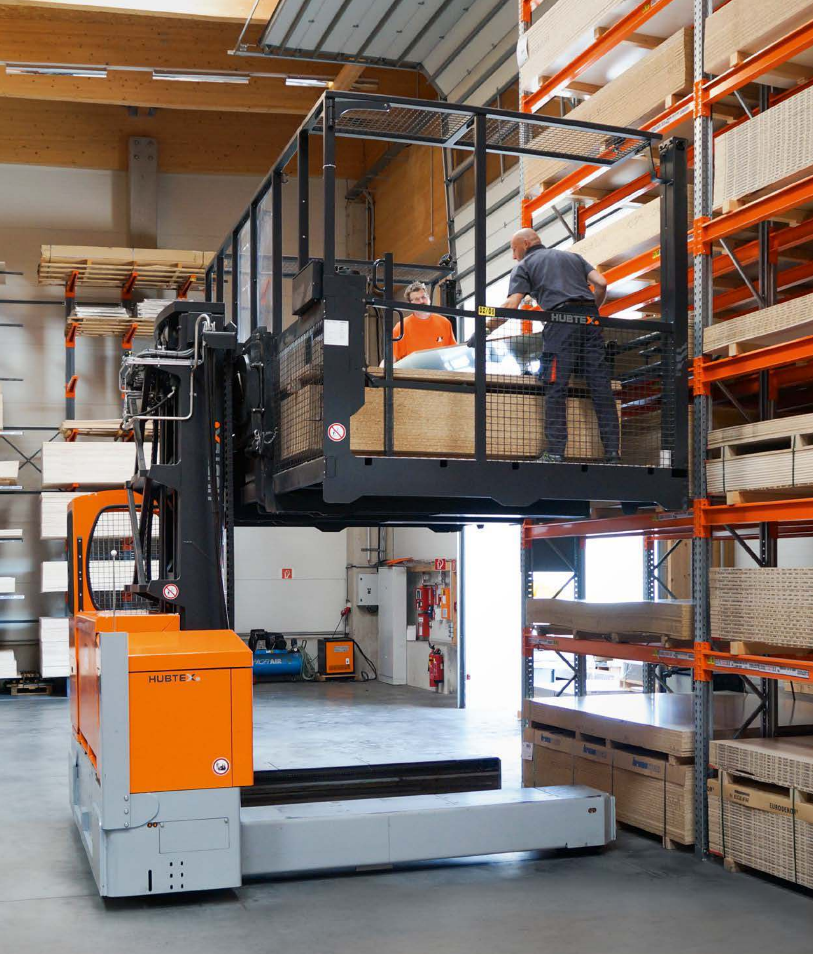
Multidirectional sideloader with detachable order picking platform
